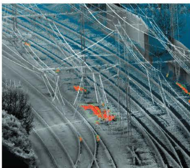
Automated detection (in red) and measurement (green bounding box) of objects which may be unintentionally left on the track following repair work
