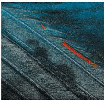
Automated detection (in red) and measurement (green bounding box) of objects which may be unintentionally left on the track following repair work
